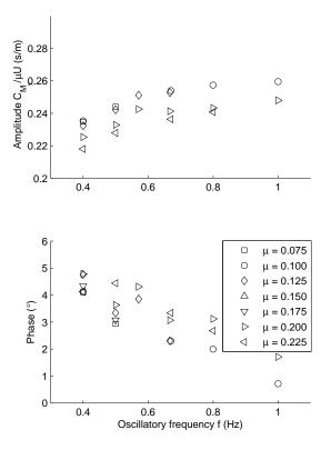
Figure 3: Effect of the oscillatory frequency and current number on the amplitude and phase response of the out-of-plane blade root bending moment, for single frequency planar oscillations about  $\lambda = 4.5$ .
