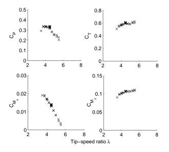
Figure 2: Clockwise from top left: rotor power, thrust, outof-plane and in-plane blade root bending moment coefficients, as a function of tip-speed ratio, for steady flow velocities at a constant rotational speed of  $\Omega = 96$ rpm.
