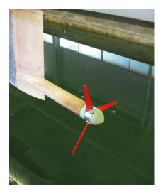
Figure 1: Photo showing the rotor and blades prior to installation on the carriage
