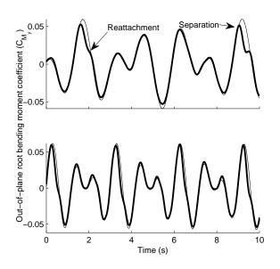
Figure 5: Time histories of the out-of-plane root bending moment for multi-frequency oscillations with frequency combinations of f = 0.4, 0.67Hz (upper) and f = 0.67, 1Hz (lower). The Current number of each component is  $\mu = 0.15$ , and the reconstruction using the transfer function is shown by the solid line.
