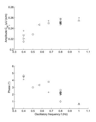
Figure 4: Amplitude and phase of the out-of-plane root bending moment for multi-frequency cases about  $\lambda = 4.5$ , where each frequency component has a current number of  $\mu = 0.1$ . Each case is depicted by a separate set of symbols, and the estimates from the single frequency oscillatory tests are shown by the (+) symbol.
